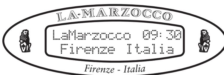
The digital display (display) is a backlit display capable of displaying 2 lines of 16 characters. The display enables the operator to interact with the espresso machine to visibly change parameter values. The display also provides valuable information to the operator. There are several warnings that can be displayed to alert the operator of an unusual condition or a fault. Additionally, simple messages are displayed alerting the operator that an action has been started.
