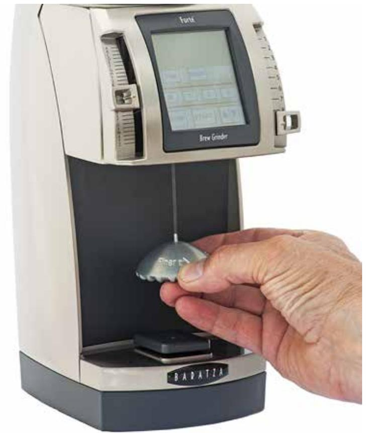
Use the burr calibration tool while the grinder is running.
